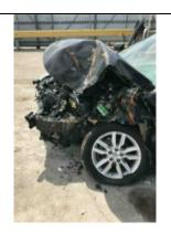
1043. On April 10, 2019, an inspector for Toyota USA inspected the wreckage of this vehicle. The EDR data recovered from the Avalon had no record of the crash. This was a sign of ASIC EOS.
