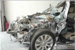
875. In or before October 2015, FCA sent ZF Automotive USA, ZF Electronics USA, and ZF Passive Safety USA the DS84 ACU retrieved from this 2012 Chrysler 200. FCA informed ZF Automotive USA, ZF Electronics USA, and ZF Passive Safety USA that the airbags did not deploy in the Chrysler 200 during a crash and requested a download and inspection of the DS84 ACU.
