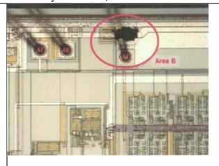
k. A decapsulation analysis from no later than the summer of 2018 of a DS84 ASIC that malfunctioned in a Toyota vehicle that crashed with no airbag deployment (pictured below as produced by Toyota).
